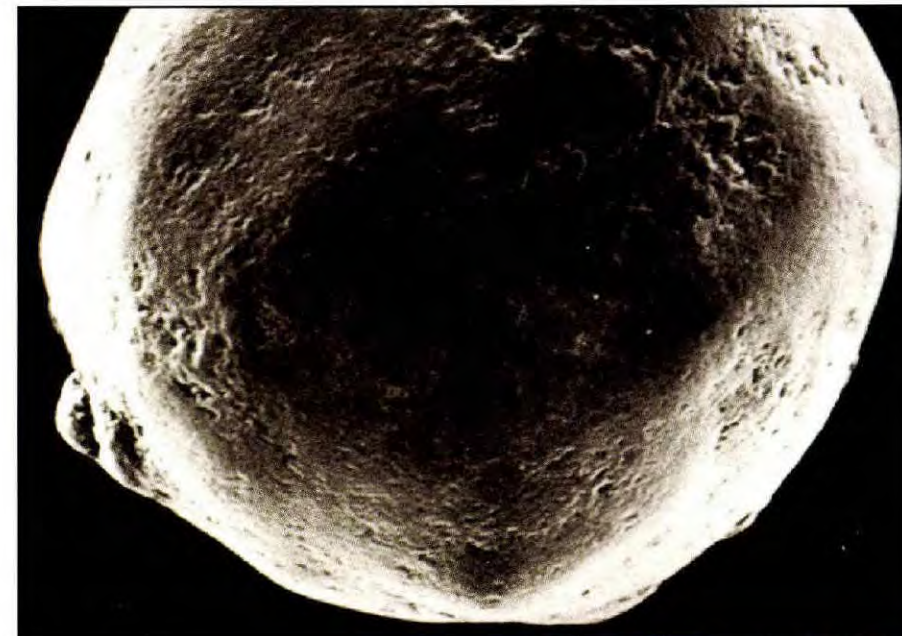
Layered pellet with micronized drug suspended in binder solution
