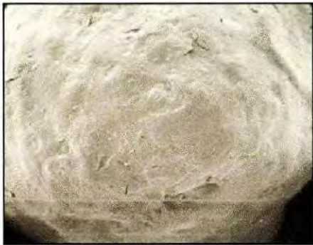
Wurster HS latex coated pharmaceutical (particle size < 150 μm)
