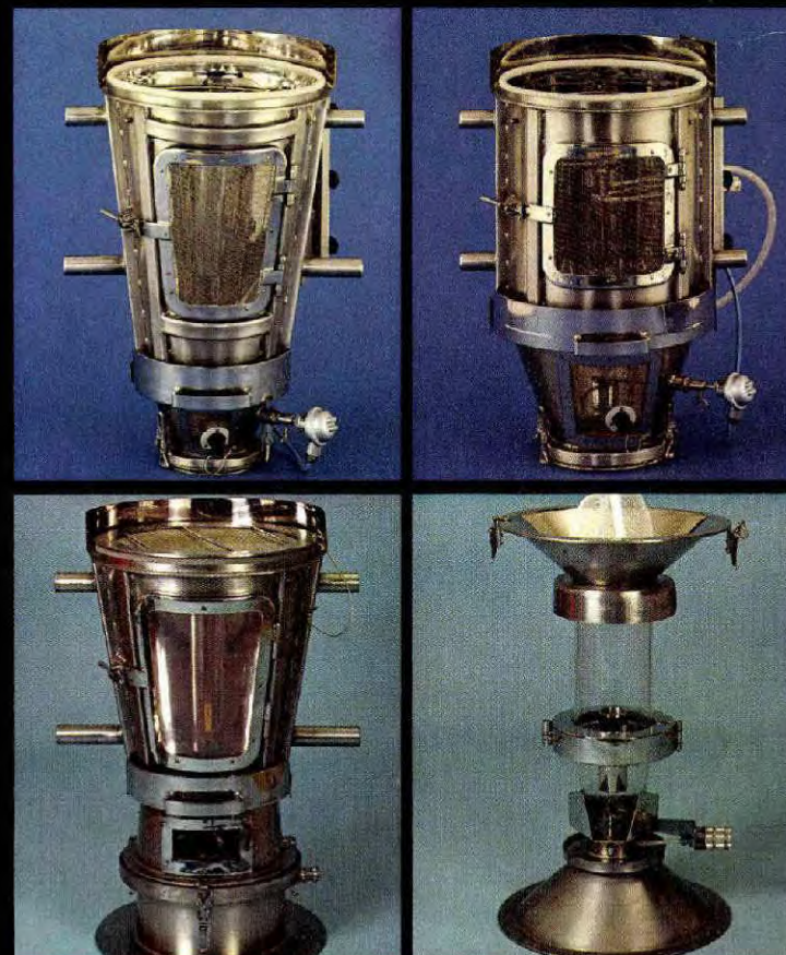
The various inserts of the changeable Glatt Fluidized Bed system.
