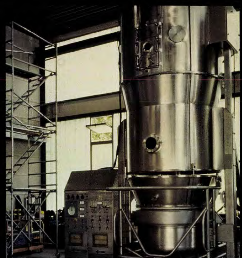
Final inspection of World's largest Fluid Bed Granulator/Dryer installation at Glatt, prior to shipment.
