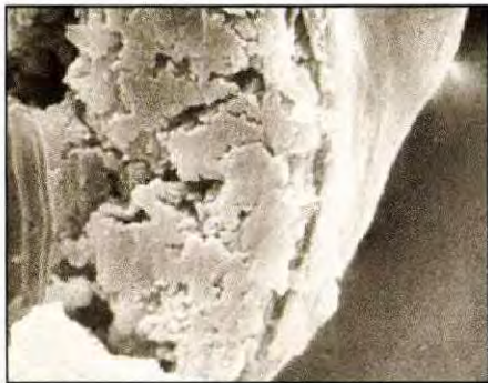
Wurster HS latex coated pharmaceutical (particle size < 150 μm) (cross-section)
