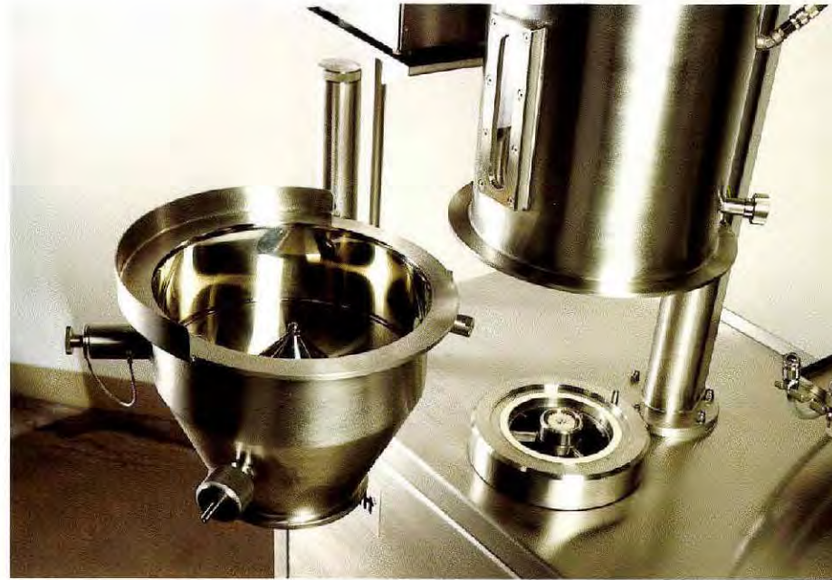
Rotor insert Easy handling with swivel device
